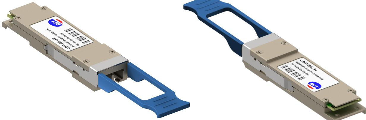
RiT QSFP-LR4-40G Compatible 40GBASE-LR4 QSFP+ transceiver provides 40G throughput up to 10km over single-mode fiber (SMF) using a wavelength of 1270nm to 1330nm via an LC Duplex connector.
